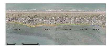
For Units 1, 3a, 3b and 4, we will be placing large rocks along the estuary edge to create an armoured rock revetment. The size of the rocks we'll be using means they won't easily move out of place in a big storm. In some places we'll be putting the rocks over existing structures. In other places we may need to remove excess material so that we end up with a consistent estuary edge that also looks good.
