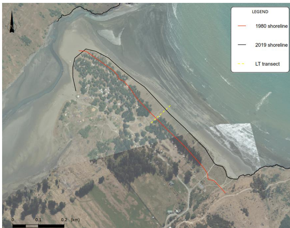
Figure 4.43: Example of shorelines used to assess long term trends in Okains Bay. Approximately 23 m of accretion measured between 1980 and 2019.
