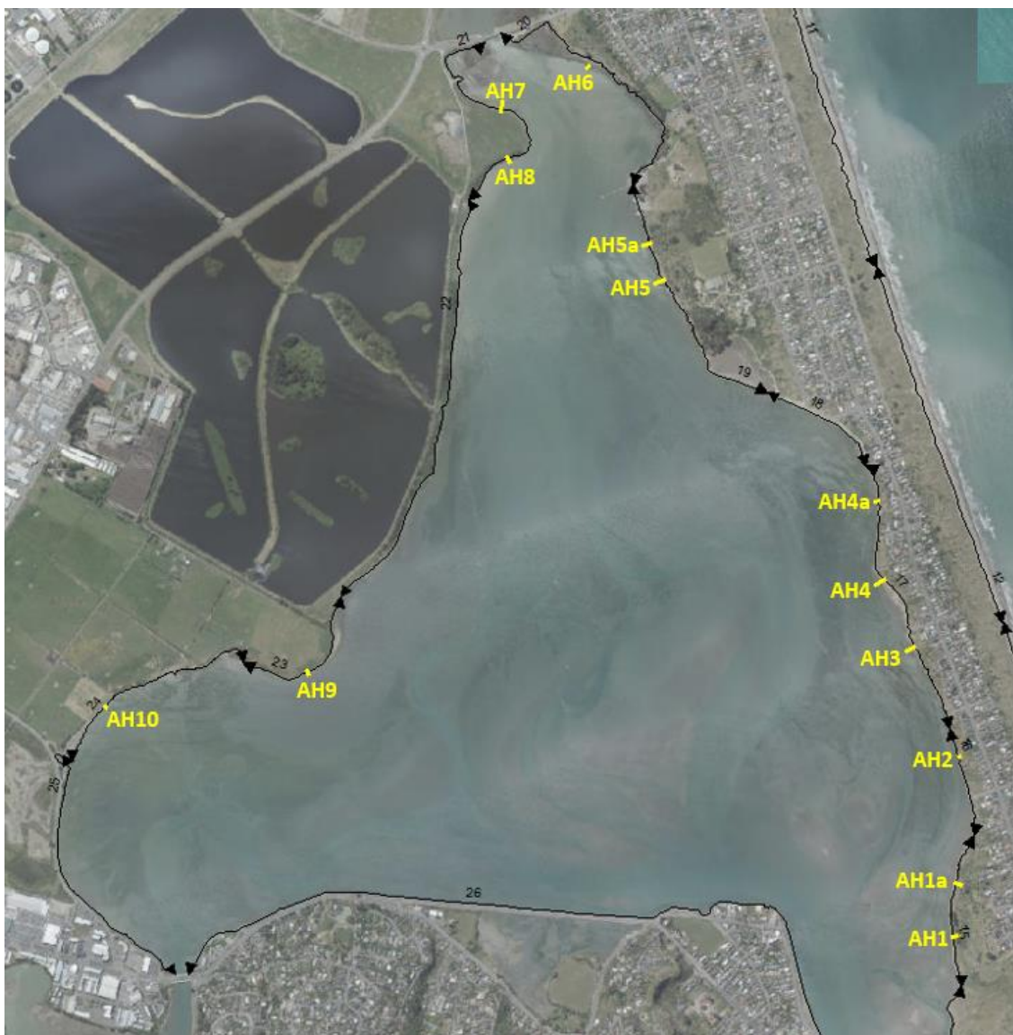
Figure 4.30: Location of transects used to assess the long term trends around the Avon-Heathcote estuary.
